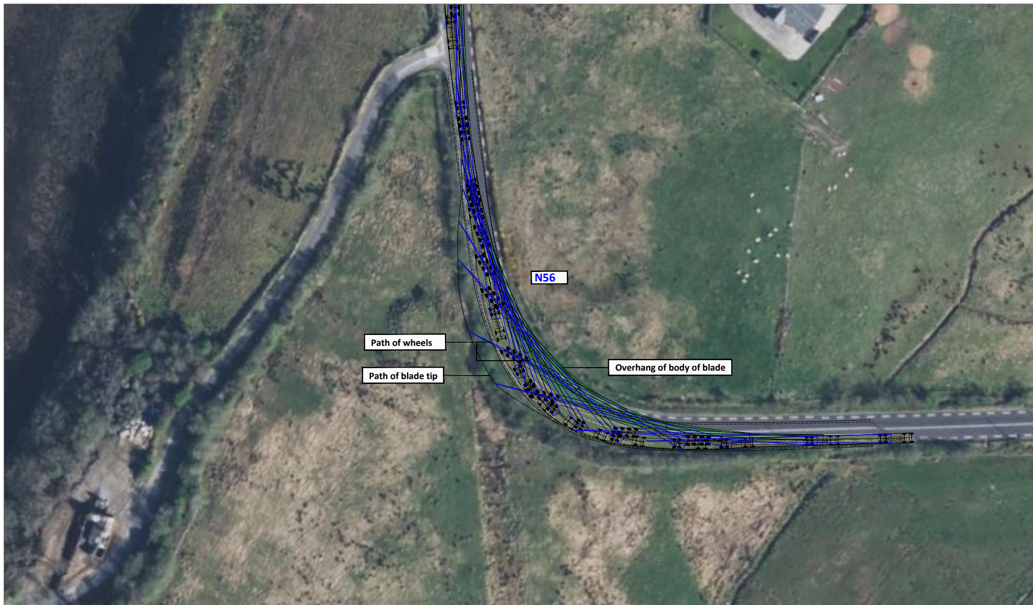
Figure 15-9 Location 5 - Bend on N56 between Bruckless and Beaugreen, blade extended artic (65.2m blade)
