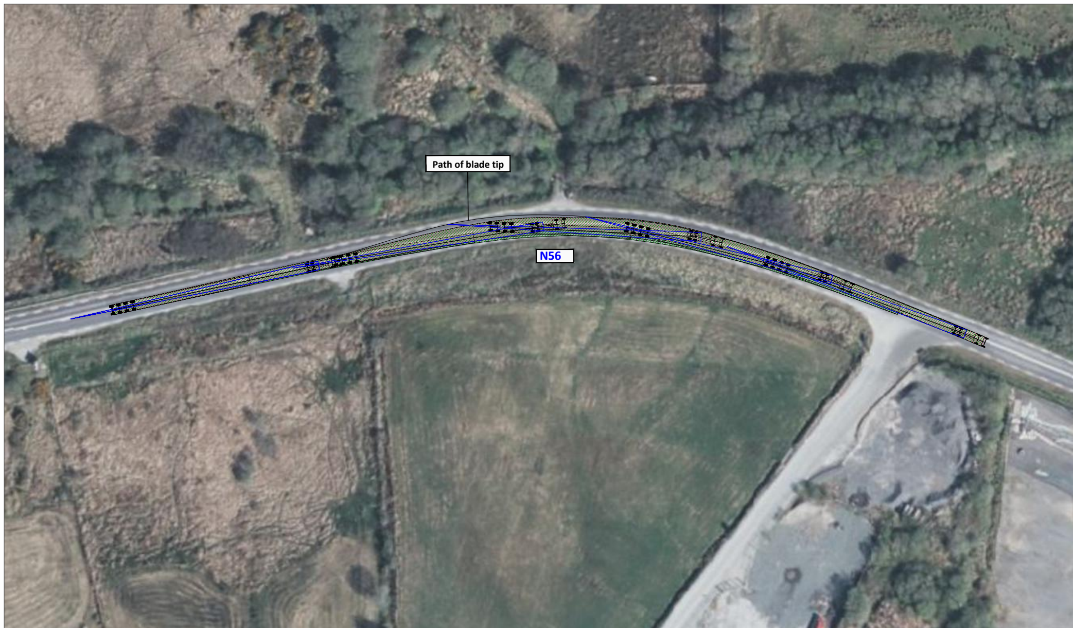
Figure 15-5 Location 1 - Bend on N56 east of Straleeney, blade extended artic (65.2m blade)
