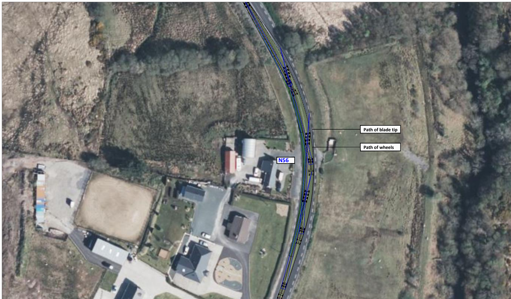
Figure 15-6 Location 2 - Bend on N56 north of Castlereagh, blade extended artic (65.2m blade)
