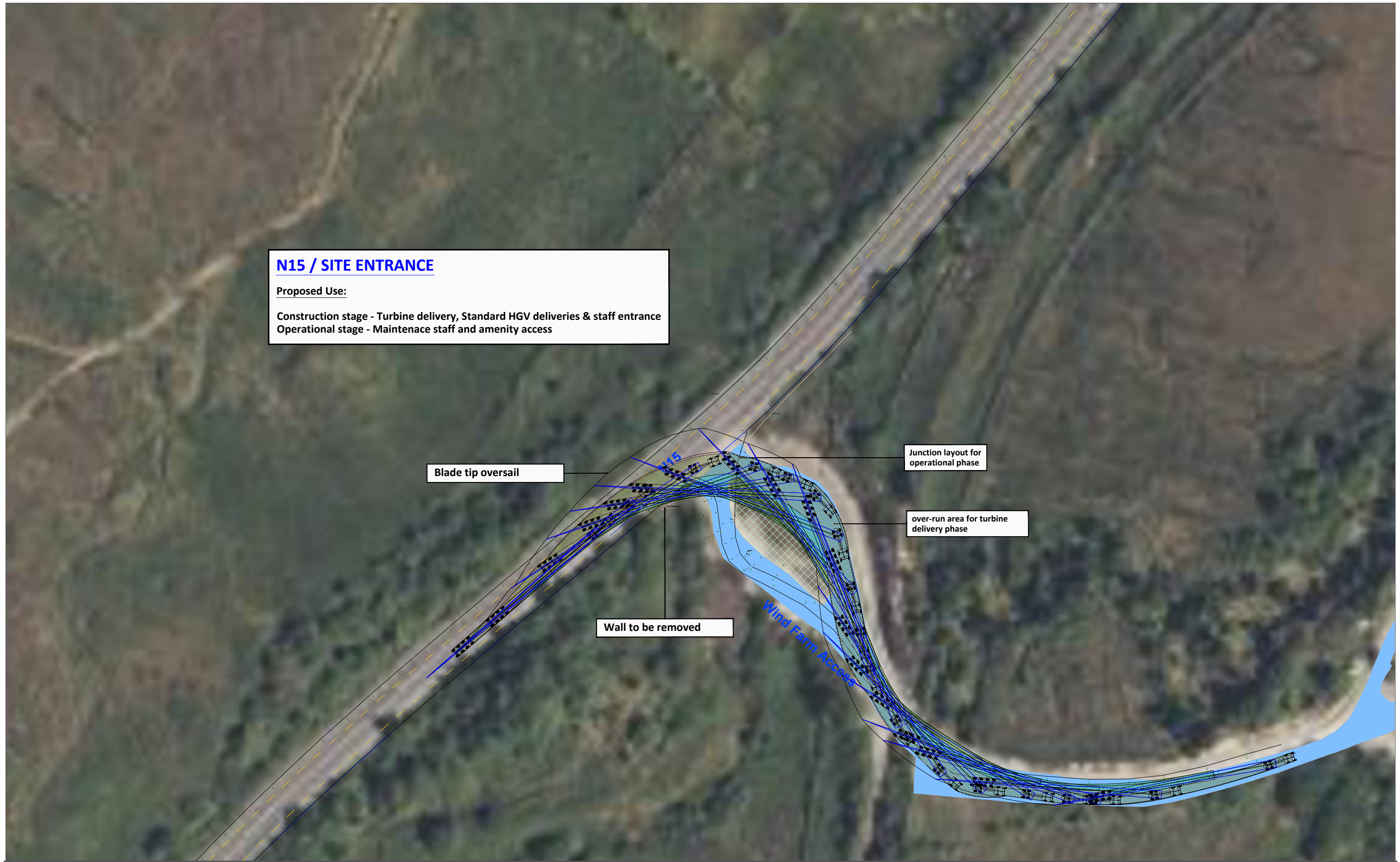
Figure 15-17 Location 10 - Access junction on N15, blade extended artic
