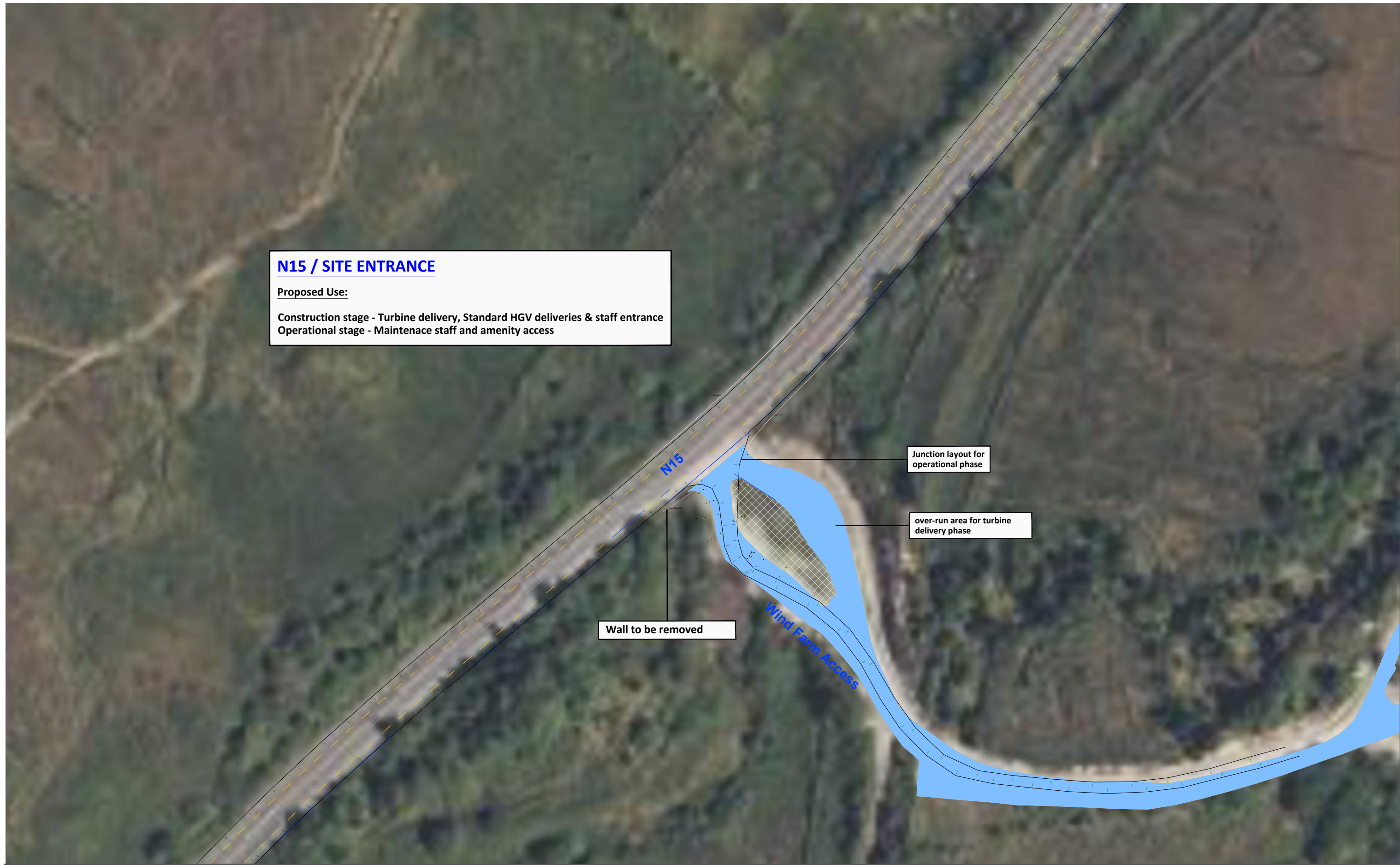
Figure 15-14 Location 10 - Access junction on N15, junction layout
