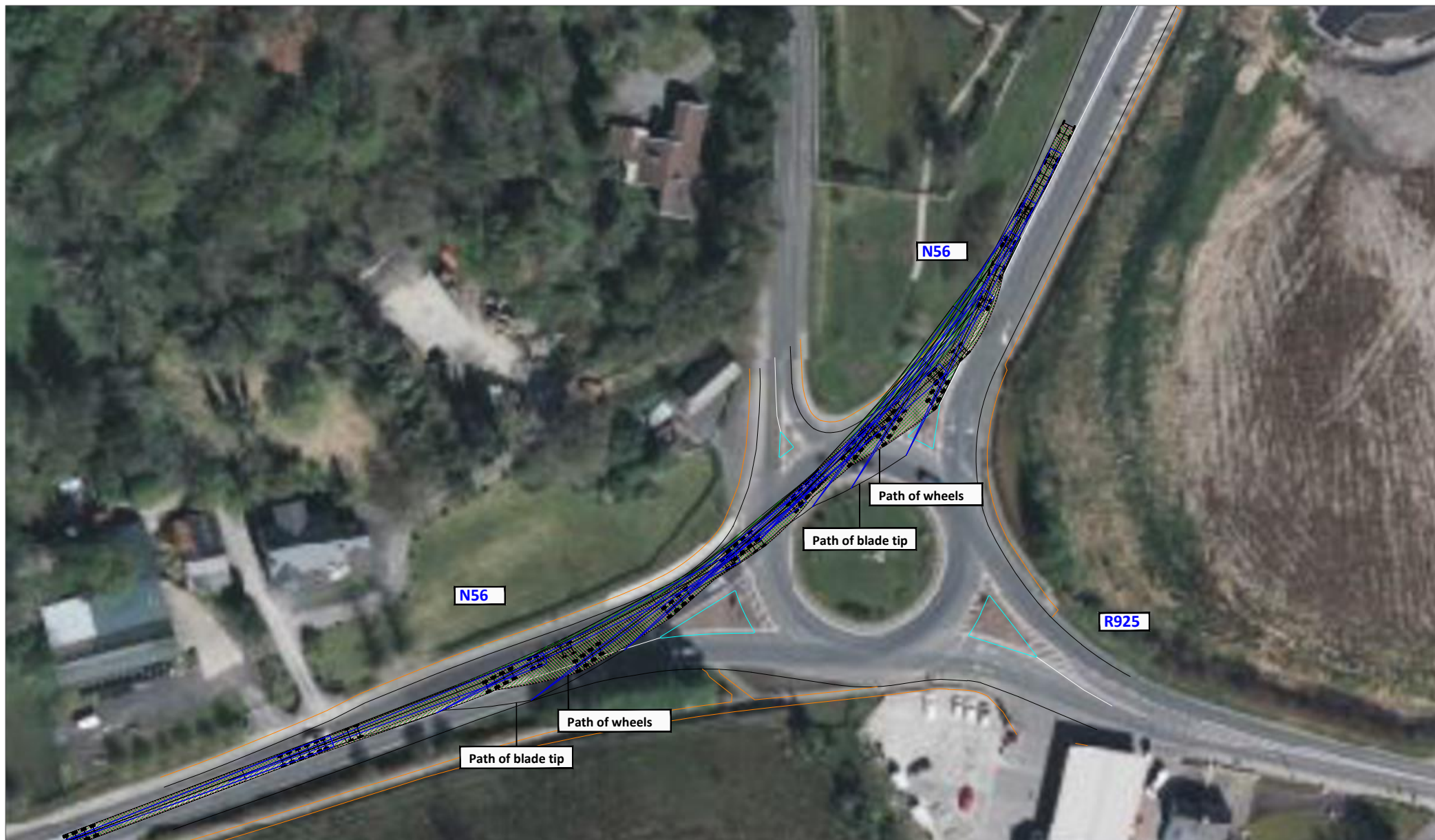
Figure 15-12 Location 8 - N56 / R925 roundabout, blade extended artic (65.2m blade)
