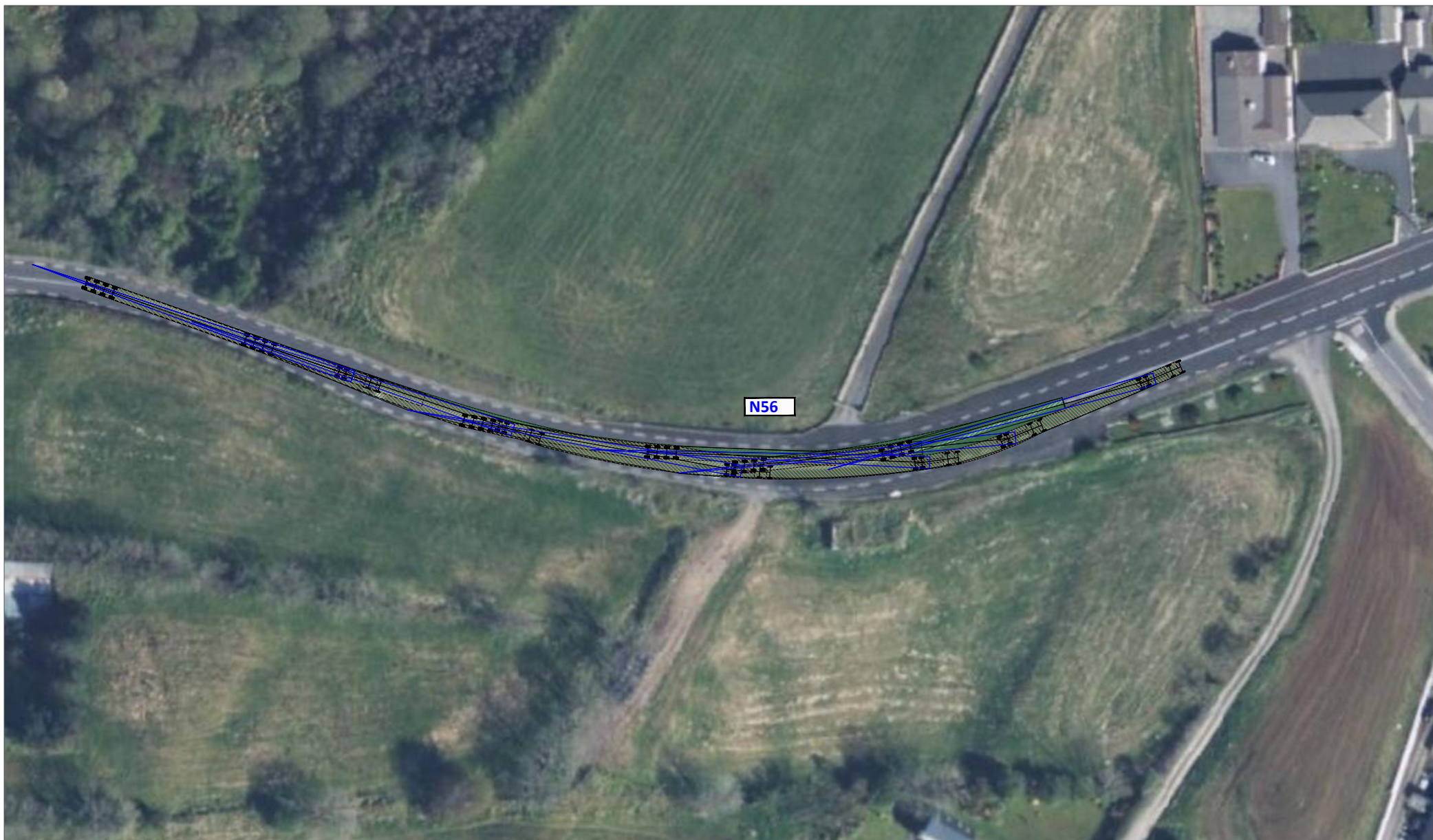
Figure 15-10 Location 6 - Bend on N56 west side of Dunkineely, blade extended artic (65.2m blade)
